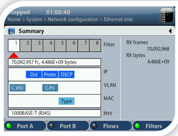
Packet Time Protocol: PTP / IEEE 1588v2 support decoding PTP support / generation using Master or Slave clock Master Clock operation on each port using internal or external clock reference
