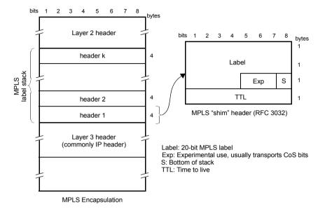
Figure 4.4 MPLS "shim" header format. The label is usually inserted between layer-2 and layer-3 headers.
