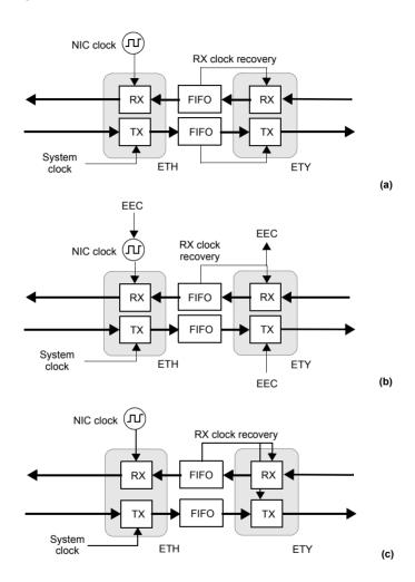
Figure 10.2: Ethernet synchronization models: (a) Conventional Ethernet. There are at least two clock domains. The transmitter and the receiver are in different clock domains (b) Synchronous Ethernet. All clocks are slaves of the EEC. The RX recovered clock could be used as an input for the EEC. (c) 1000BASE-T slave. The TX clock is always an slave of the RX clock.
