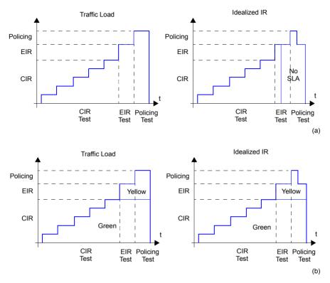
Figure 7.8: Typical CIR, EIR and Policing tests in colour-aware and non colour aware services: (a) No colours are defined in the interface. Some traffic may be degraded if CIR < IR < EIR because quality of service is not guaranteed for excess traffic. If IR > EIR some traffic will be lost due to the action of the policing filter. (b) Coloured interface: Yellow traffic does not have quality of service guarantees but SLA is meet for Green traffic as long as the IR remains smaller than the CIR.
