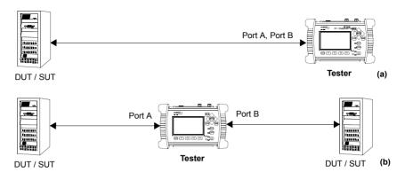
Figure 2.1: Basic connection setup for Ether.Genius, Ether.Sync and Ether.Giga testers: (a) Ethernet and IP endpoint operation modes. (b) Ethernet / IP through mode.
