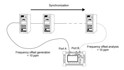
Figure 10.3: If Synchronous Ethernet is used for transmission of timing signals, network elements in the chain should be transparent to offset generation at is input and therefore any frequency offset should be recovered at the output of the chain.
