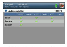
Figure 2.4: Albedo Ether.Genius / Ether.Sync / Ether.Giga auto-negotiation results panel.
