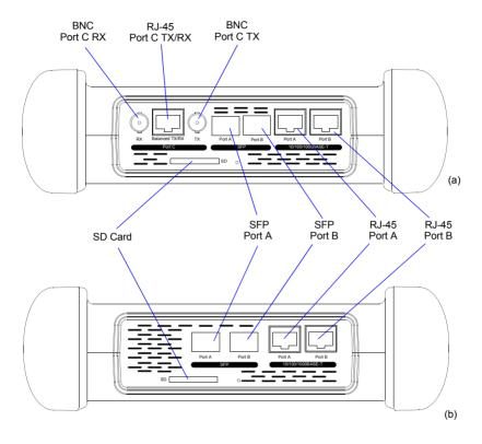
Figure 1.2: Test connector panel. Connection to the DUT / SUT is done in this panel: (a) Ether.Genius, Ether.Sync. (b) Ether.Giga
