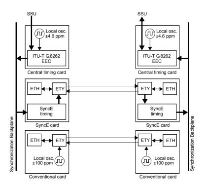
Figure 10.2 Synchronous Ethernet Architecture and comparison with conventional Ethernet
