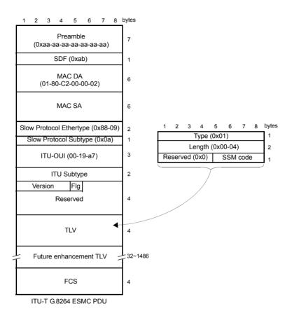
Figure 10.1: Ethernet Synchronization Message Channel (ESMC) protocol data unit.
