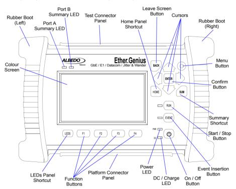
Figure 1.1: Ether.Genius front view. The tester presents results by means a colour screen and the LEDs. The configuration is performed through the keyboard.
