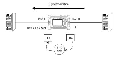
Figure 10.4: With the help of Ether.Genius or Ether.Sync it is possible to generate frequency offset in pass-through mode to stress the network.
