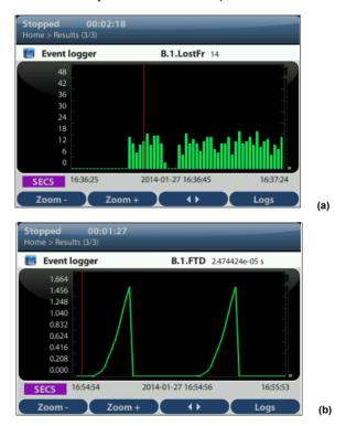
Figure 5.5: Ether.Genius / Ether.Sync / Ether.Giga detailed view of events: (a) Bar diagram (frame loss), (b) line diagram (frame delay).
