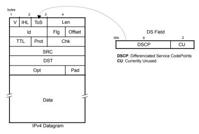
Figure 4.6: IPv4 datagram structure.
