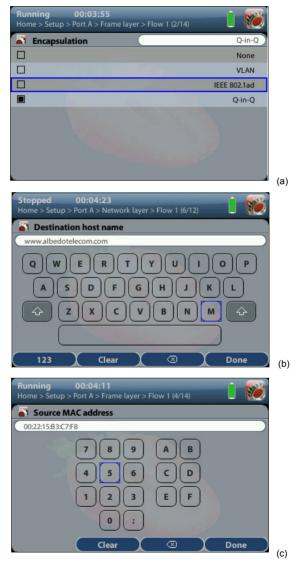
Figure 1.6: Different kinds of configuration panels: (a) Selection list, (b) Alphanumeric keyboard, (c) Numeric keyboard.
