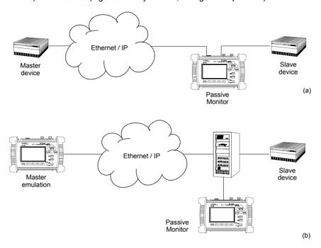
Figure 9.4: Connection of Ether.Genius / Ether.Sync to the network in PTP *Passive monitor* mode: (a) Connection in pass-through mode (IP through operation mode). (b) Connection in endpoint mode (*Ethernet endpoint* or *IP endpoint* operation modes).
