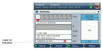
Figure 2.2: Laser on indication in the Ether.Genius / Ether.Sync / Ether.Giga Summary panel.
