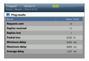
Figure 8.1: Ether.Genius / Ether.Sync / Ether.Giga Ping results panel.
