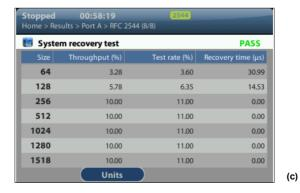
Figure 7.2: RFC 2544 test results: (a) Frame loss result table, (b) Back-to-back frames result table, (c) System recovery time results table.
