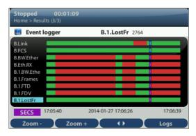
Figure 5.4: Ether.Genius / Ether.Sync / Ether.Giga event logger panel. This panel traces all events previusly selected from the event filter.
