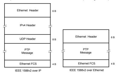
Figure 9.2: IP and Ethernet encapsulations for PTP messages.
