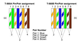
Figure 3.1: T-568A and T-568B wiring standards. Pair numbering (1, 2, 3, 4) is a way to identify pairs in the cable and is not to be confused with MDI numbering (MDI-0, MDI-1, MDI-2, MDI-3).
