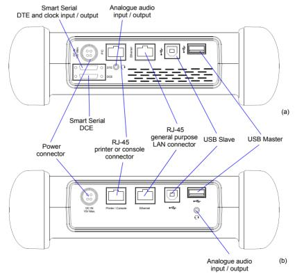
Figure 1.3: Platform connector panel. This panel includes connectivity to USB devices, Ethernet networks and power source: (a) Ether.Genius, Ether.Sync. (b) Ether.Giga.
