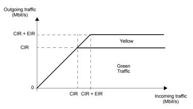
Figure 7.6: The amount of traffic that crosses an admission control filter. Graphics represent steady states, traffic is usually allowed to be greater than the CIR and EIR for short periods of time. Traffic delivery is guaranteed if the rate is smaller than the CIR. Excess traffic (EIR traffic) is delivered as well, but it is marked as low priority and usually discarded first if congestion occurs.
