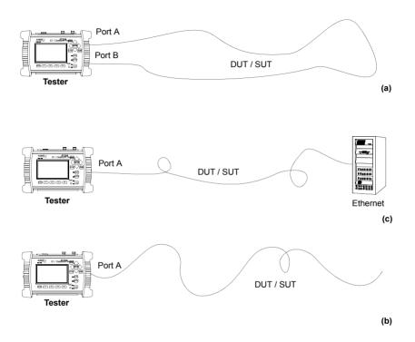
Figure 3.2: Basic connection setup for Ether.Genius, Ether.Sync and Ether.Giga testers: (a) Port A - Port B closed loop, (b) Port A connection with remote link, (c) Port A connection without link.
