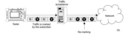
Figure 7.4: (a) Non-color-aware service. It the service provider is wiling to implement different transmission priorities for this service, marking will have to be carried out by the access network by means some traffic classification algorithm. (b) In a color-aware service subscribers mark their own traffic from the beginning. The service provider may remark some traffic depending on the traffic acceptance algorithm.
