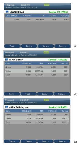
Figure 7.7: CIR, EIR and policing test results as presented by Ether.Genius / Ether.Sync / Ether.Giga.
