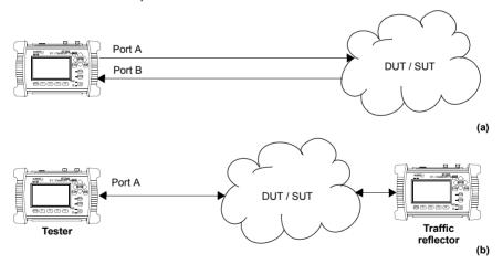
Figure 2.3: Connection setup for one-way and two-way tests: (a) One-way test, the test pattern leaves the tester in port A and it is received in port B. (b) Two-way test, the test pattern leaves in port A and it is received in the same port A.
