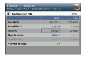
Figure 4.3: Albedo Ether.Genius / Ether.Sync / Ether.Giga bandwidth profile configuration panel.
