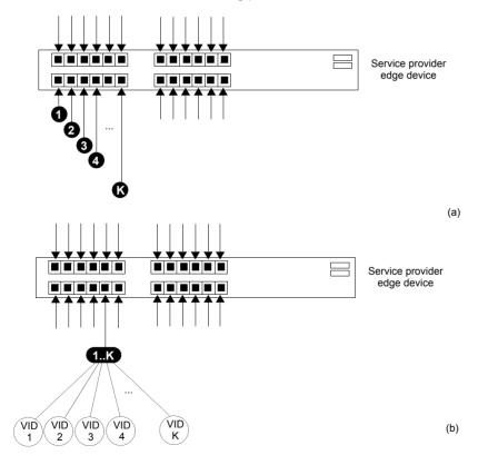
Figure 7.3: (a) Port based Ethernet service, one service per port. (b) Ethernet service multiplexing based on service delimiting markers like the VLAN tag.
