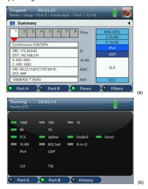
Figure 1.7: Special panels: (a) Summary panel, (b) LEDs panel.
