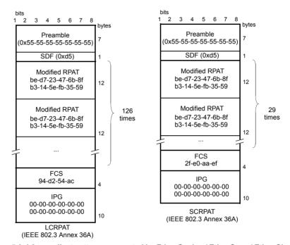
Figure 5.6: L2 compliant patterns supported by Ether.Genius / Ether.Sync / Ether.Giga.
