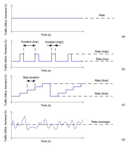
Figure 4.4: Bandwidth profiles for Albedo Ether.Giga / Ether.Genius / Ether.Sync testers: (a) Continuous traffic generation, (b) Periodic burst generation, (c) Ramp generation, (d) Random traffic generation with Poisson probability distribution.
