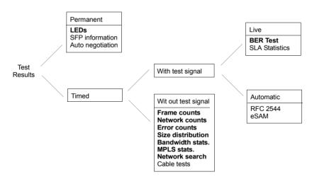
Figure 5.1: Statistics and counts available in Ether.Genius / Ether.Sync /Ether.Giga.
