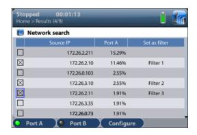
Figure 5.2: Ether.Genius / Ether.Sync / Ether.Giga network search capability
