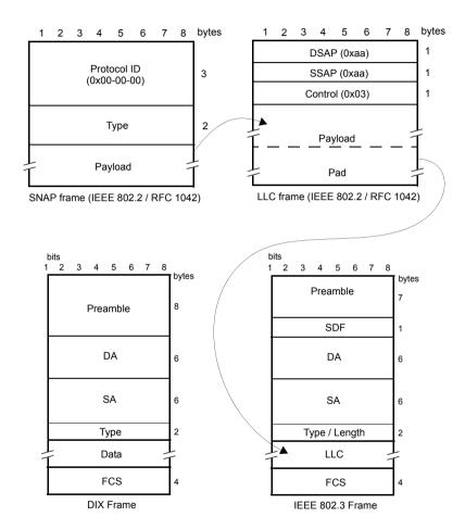
Figure 4.1: MAC frame structure: IEEE 802.3 and DIX
