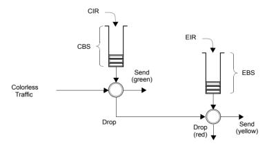
Figure 7.5: Two-rate Three color marker (trTCM), policing algorithm.
