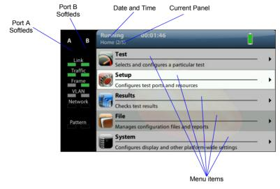
Figure 1.4: Ether.Genius / Ether.Sync / Ether.Giga Home panel.
