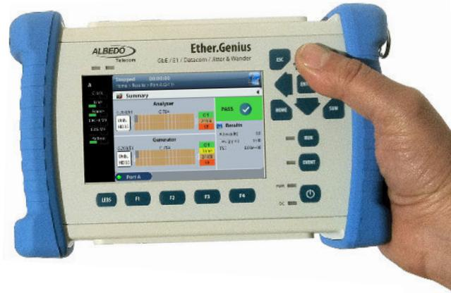
**ALBEDO Ether10.Genius** is a multitechnology Ethernet tester that includes a Rubidium clock. It is ideal to install and measure advanced services based on GbE, SyncE, PTP, T1/E1, 1 pps, ToD, C37.94, Datacom, OWD
