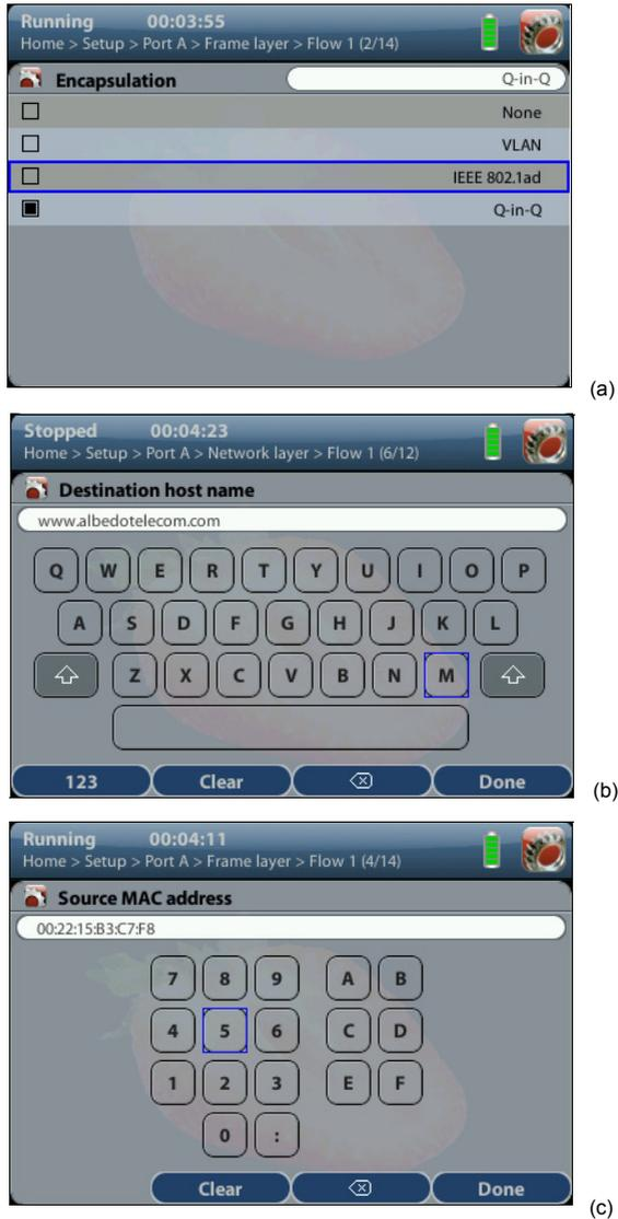
Figure 1.6: Different kinds of configuration panels: (a) Selection list, (b) Alphanumeric keyboard, (c) Numeric keyboard.
