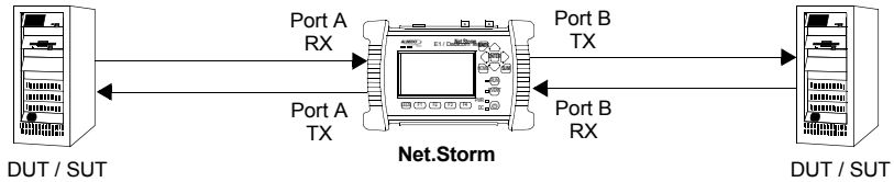
Figure 2.1: Bidirectional impairment generation with ALBEDO Net.Storm connected in pass through mode
