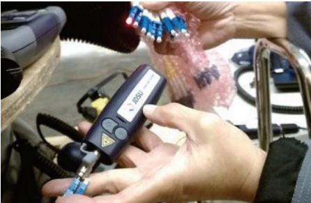
A JDSU FFL-050 VFL detects bends, breaks, and fiber continuity.
