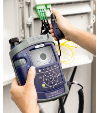
SmartClass Fiber system with integrated power meter and patch-cord microscope
