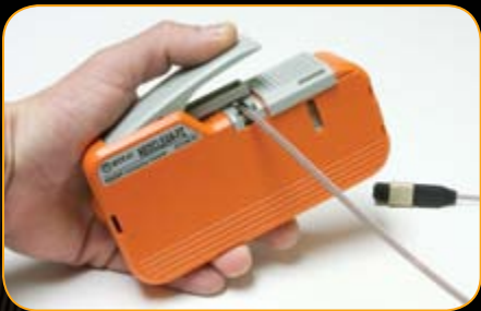
Cleaning PRIZM® LightTurn® connector
