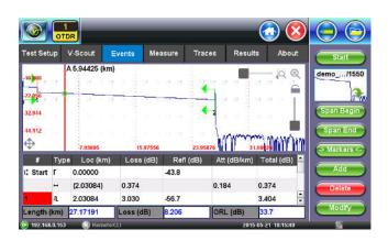
The MTTplus-410 OTDR employs specialized techniques developed from decades of experience to locate and measure connectors, splices, optical splitters and macro-bends.
