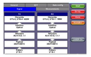
The transmitter and receiver can operate independently, or they can be coupled depending on test setup. Framed signals can be equipped with unstructured or structured payloads with selected test pattern filling the entire test payload (Bulk) or a structured payload (SDH/SONET framed client signal) with or without PDH/DSn multiplexed clients. Layer-based graphical configuration interface allow users to build the test signal in a logical layer by layer sequence
