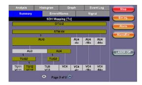
PDH/DSn client can be multiplexed and mapped into SDH/SONET, which in turn can be mapped and multiplexed into OTN using bit-synchronous or asynchronous modes. In synchronous mode the Optical Payload Unit (OPU) clock is derived from the mapped client signal while in asynchronous the OPU clock is independent.
