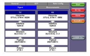
The transmitter and receiver can operate independently, or they can be coupled depending on test setup. Framed signals can be equipped with unstructured or structured payloads with selected test pattern filling the entire test payload (Bulk) or a structured payload (SDH/SONET framed client signal) with or without PDH/DSn multiplexed clients.
