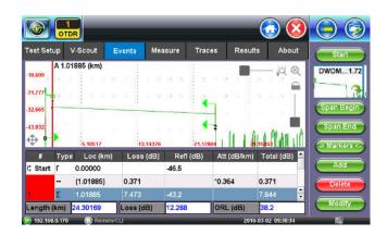
The DWDM OTDR employs specialized software algorithms developed from decades of experience to measure fiber attenuation including anomalies such as connectors, splices, and macro-bends. Precise location and analysis of ROADM network elements is also supported.
