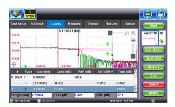
The OTDR module employs specialized software and algorithms developed from decades of experience to locate and measure connectors, splices, optical splitters and macro-bends.
