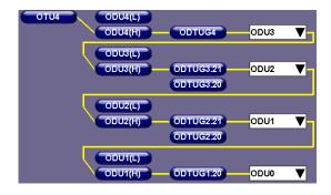
OTU4 multi-step mapping/multiplex structures
